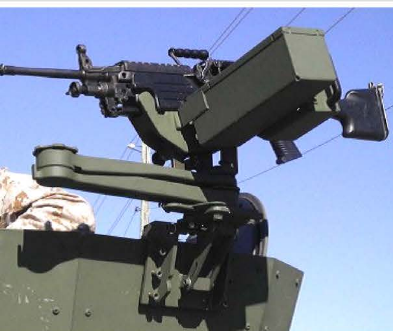
Clamp-on 30 bolted on the vertical shield surface (left); 'B' Pillar Clamp-on bolted on the roll bar (right)
